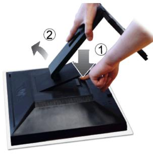
After placing the monitor panel on a soft cloth or cushion, complete the following steps to remove the base.
