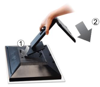
After placing the monitor panel on a soft cloth or cushion, complete the following steps to attach the base.
